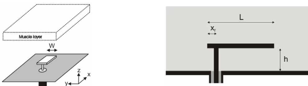
Figure 1: 3D configuration (left) and cross-section (right) of the patch antenna configuration and a cross-section, with the dimensions that are varied. The "Muscle layer" was present only in the setups that were used to investigate influence of a patient on the reflection characteristics.
